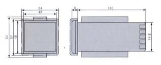
\*Double-dotted lines show the front cover conforming to NEMA 4X. The panel thickness shall be 1 to 10mm.
