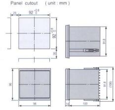
\*The panel thickness shall be 1 to 8mm.
