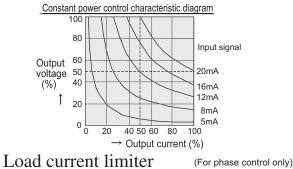
This function limits the load current value to the heater. The setting range is 30 to 100% of the rated current.
